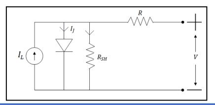
Equivalent circuit of Photovoltaic cell is shown in figure.
