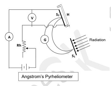
A pyrheliometer contains the following three important parts.
