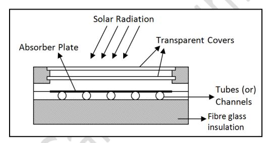
Schematic view of a flat plate collector is shown in figure. It contains four important components.
