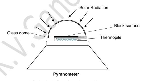
A pyranometer contains the following three important parts.
